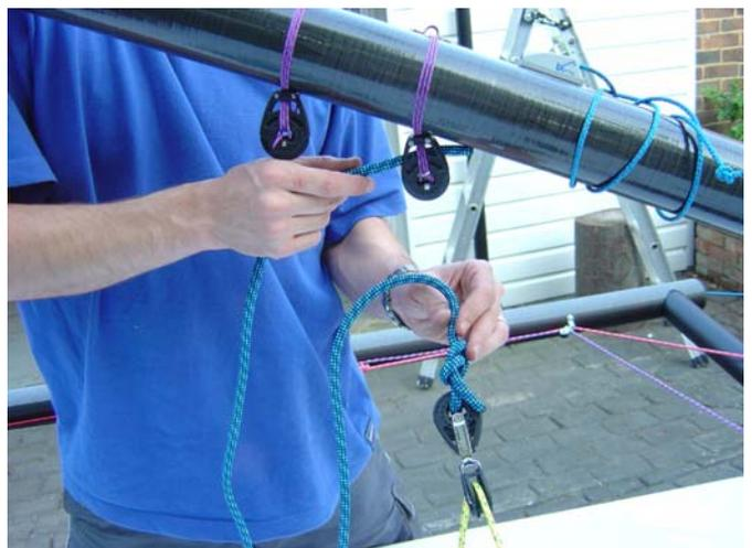
32. Rig the mainsheet starting with a knot through or around the block attached to the mainsheet bridal. The method of tying is optional. Then thread it through the front block on the boom.
