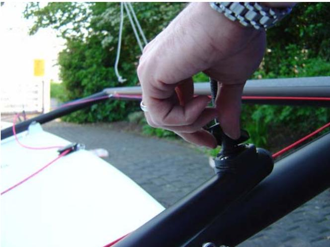
65. Clip and tape the tiller extension onto the tiller.
