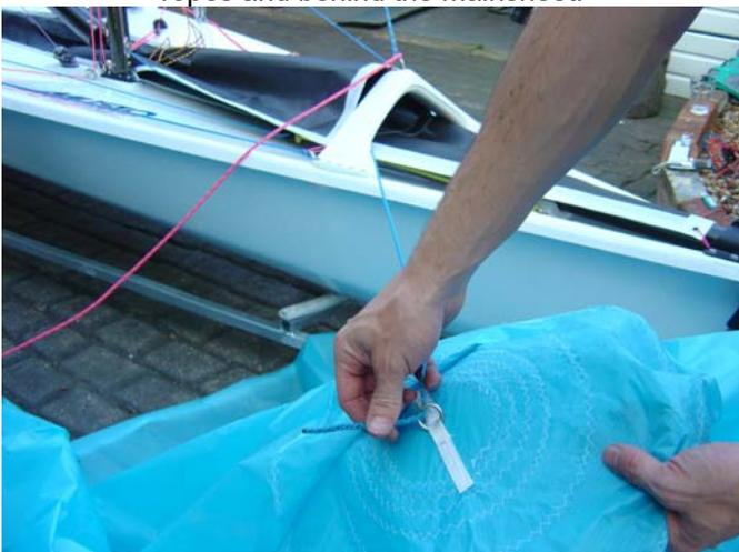
57. Un-tie the downhaul from the forestay eye (remember step 49). Make sure it is underneath the kite sheets; thread it through the ring on the kite.
