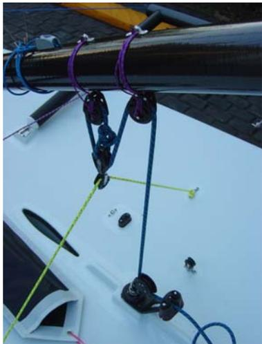
33. Then thread it through the block on the bridal then back through the aft block on the boom and through the jammer. **MAKE SURE YOU GET IT THE RIGHT WAY THROUGH THE RATCHET BLOCK,**
