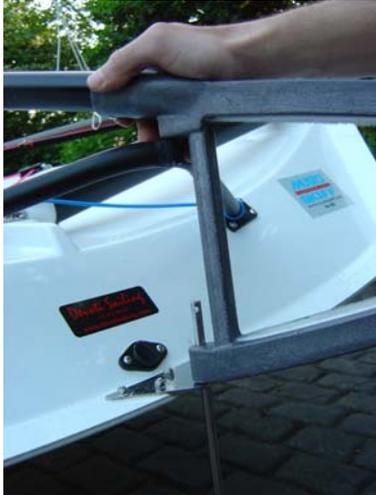
63. Offer the stock up to the pintles and insert the pin from below the bottom pintle plate
