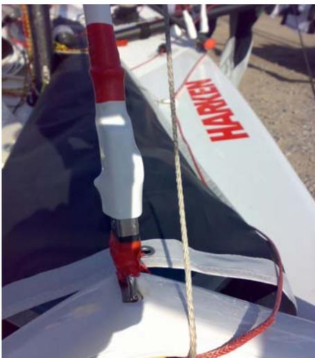
22a. Now tape or cover the chainplate AND the upper eye that the rig tensioning device was attached to, to prevent the spinnaker snagging
