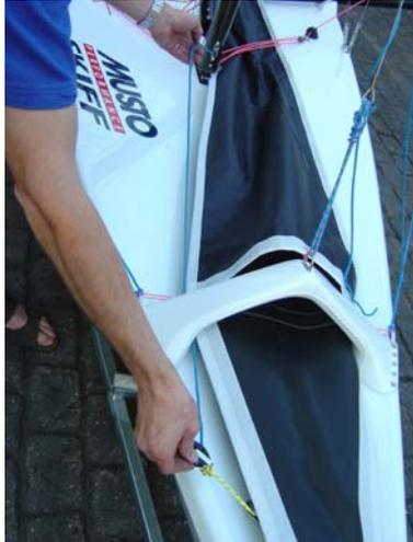
41. Take the halyard from the block exit on the front of the mast, under the chute throat and through the block attached to the pole "puller"
