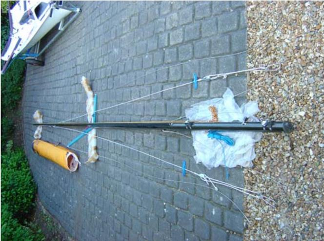
15. Before stepping the mast lay it out (on padding, so you don't scratch your new carbon mast). Check the lines and wires are not twisted. LOOK UP to check you are not going to hit anything when you raise mast, especially power lines!!
