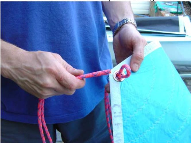
51. Then you may attach the kite sheets to the clew. There are various options for attaching the sheets, some are shown on the class website. This method shown involves finding the middle of the sheets and push the loop through
