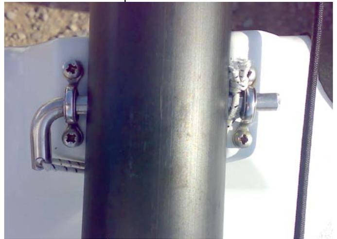
13. With the elastic between the wing and the deck eye the elastic shouldn't get knocked off and you won't lose any pins. The folded ends of the pins should preferably be away from the cockpit so that ropes don't get caught on the pin.
