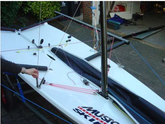
21. Attach the shroud to the outboard rig adjuster. Five holes down on the front row is a good start but check [www.mustoskiff.com](http://www.mustoskiff.com) for tuning information
