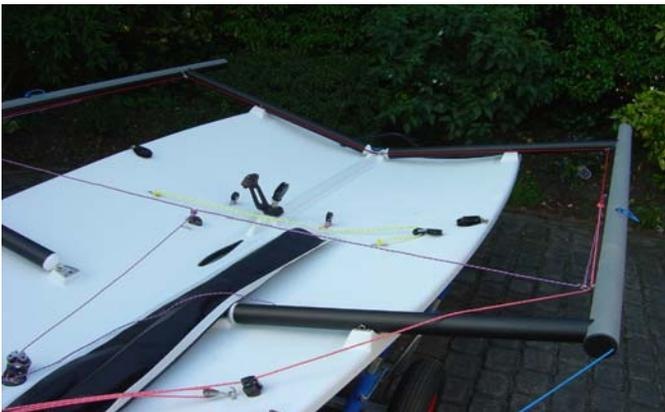
14. With the wings fitted ensure that the line for the downhaul (pink in this picture) is on top of the wing bar.
