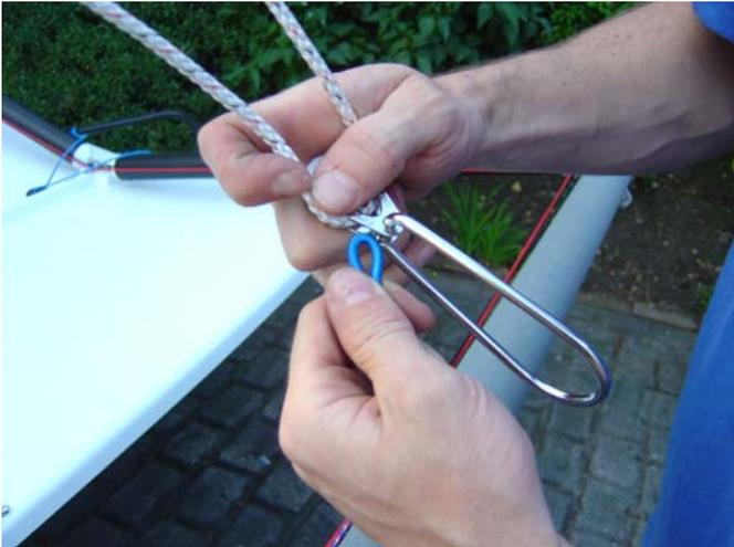
23. Now the rig is tensioned the trapezes can be connected to the elastic in the middle of the wing bar.
