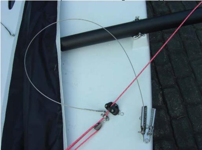
17. Attach the lower shroud to the inboard rig adjuster. Five holes down on the front row is a good start but check [www.mustoskiff.com](http://www.mustoskiff.com) for tuning information
