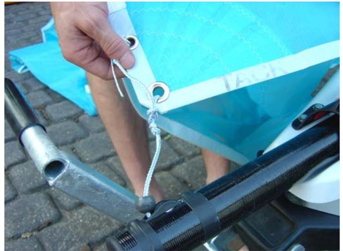
50. Roll the kite out and tie the tack on the clew line eg with a bowline.
