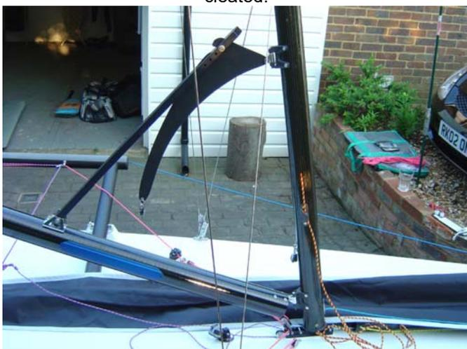
37. Locate the bolt of the other kicker bar into the slot in the lever, to link them together. Note if they will not then just adjust the height of the boom by adjusting the angle of the boom with the main halyard.
