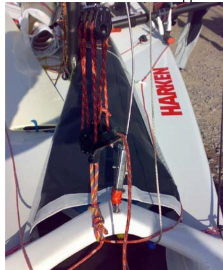
22. Now you have both shrouds and lowers are attached tension the rig using the tensioning device and then locate the lower eye (shown blue arrow in step 19) into the bow chainplate and insert the pin. Then remove the tensioning device. NOTE: Please don't over tension the rigging; call Ovington Boats if unsure on required rig tension.
