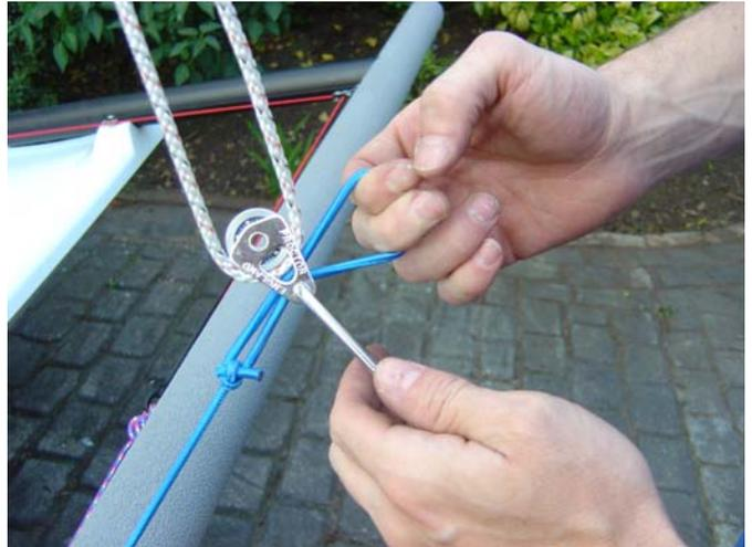
24. This can be done different ways. One option is tie a loop and pull it through the ring block.
