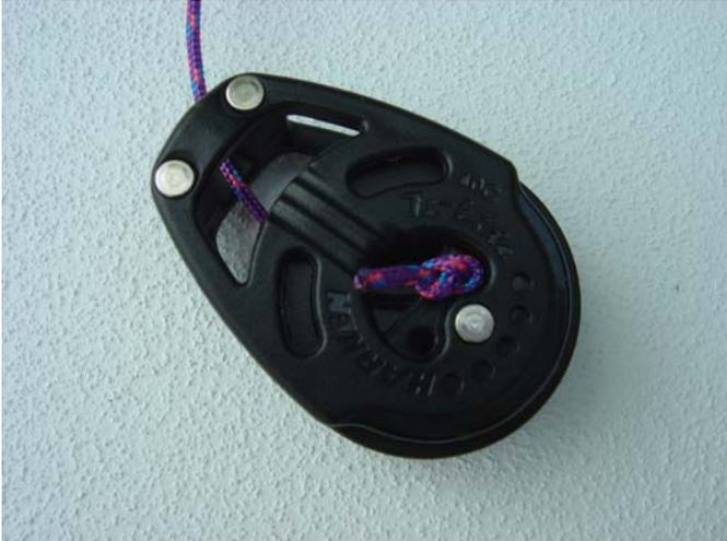
3. First - fit the Harken blocks to the boom for the mainsheet. Thread a string through the block
