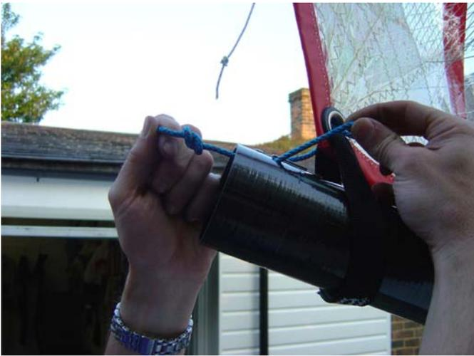
76. Back through the hole in the boom and terminate.
