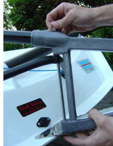
64. Insert the split ring or do up the nut at the top to hold the pin in place. Once on the stock it can be left on the boat permanently.
